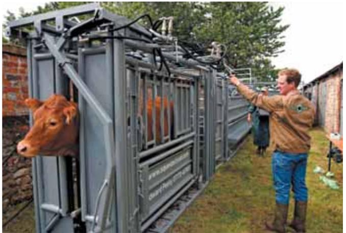
*Above right: a full system with a hydraulic Squeeze Crush.*
