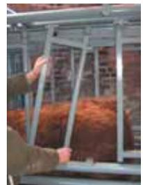
*On all Squeeze Crushes, the vertical bars click open (above left) and can be removed (above right).*
