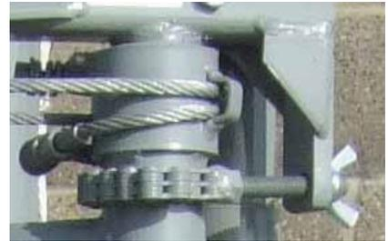
*Above: an ingenious system allows quick adjustment to enable a large bull or horned beast to enter and lock the fully opened head gate (left).*
