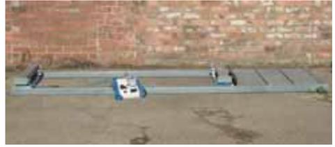
*Above: components of the weigh system: long scale base (includes section for vet gates), chute mounts, heavy-duty load bars, monitor).*
